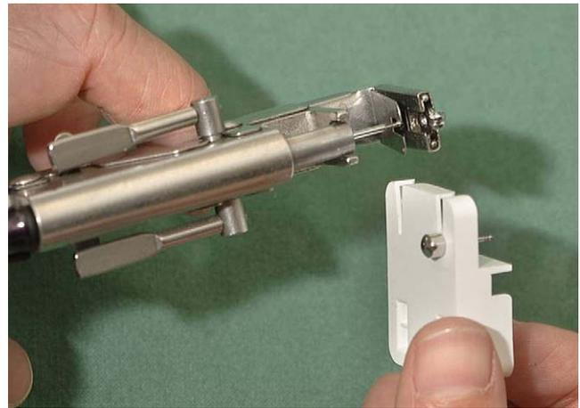
**Figure 1** Traditional open spring-loaded piercing gun US. Patent 4020848 + Caflon 1.20 mm diameter studs.
